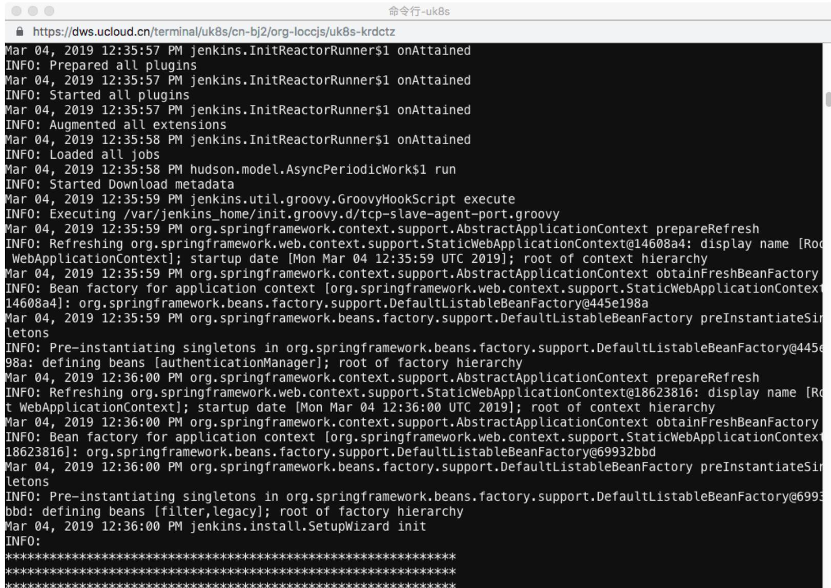
A terminal window titled "命令行-uk8s" showing the output of a kubectl command. The logs show the Jenkins initialization process, including plugin preparation, job loading, and Spring Framework context refreshes. The terminal output is as follows:
